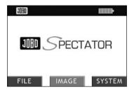
After power on, the start up screen will give you three modes to choose from. The device is also immediately in standby mode to copy files from memory cards to internal Hard Disk. If you insert a card then press 🗗 the file will be copied to Hard Disk automatically. The card type is detected as well.
